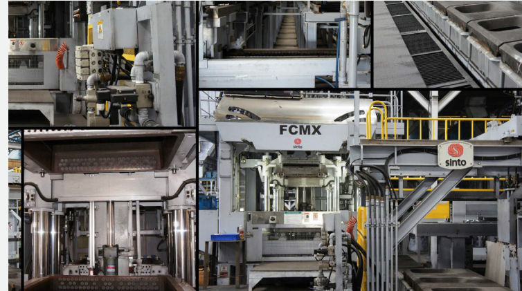
High Pressure Moulding
